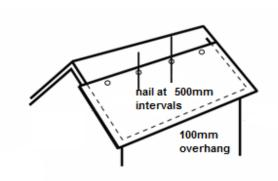
Position the first length of roof felt along the lowest part of the shed roof. Ensure that it overhangs the eaves and each gable end of the roof by 100mm.
