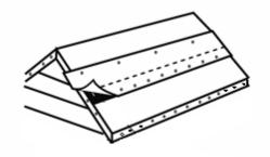
The felt will be applied in strips, with each strip overlapping the previous one by at least 75mm (see image). A final length sheet will be required along the ridge.
