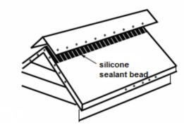
The roof should be finished with a capping sheet along the ridge. Place along the ridge of the shed so that it equally overhangs each side of the roof.
